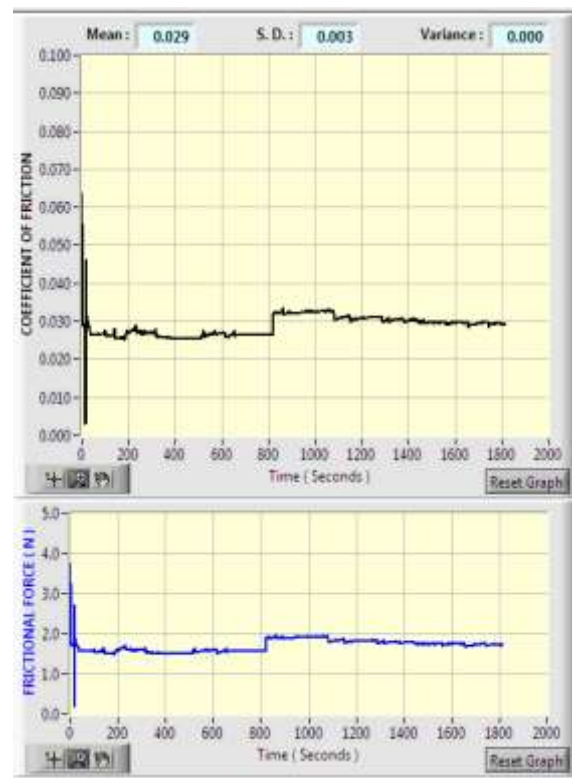
Figure 8 Coefficient of Friction & Frictional force for Trial 2 with Silicon Nitride
