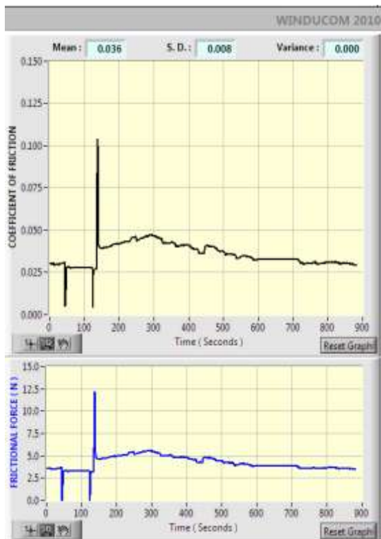
Figure 6 Coefficient of Friction & Frictional force for Trial 2 with Alumina
