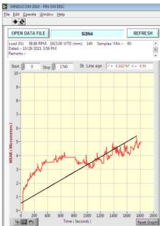
Figure 7 Wear V/s Time for Trial 2 with Silicon Nitride
