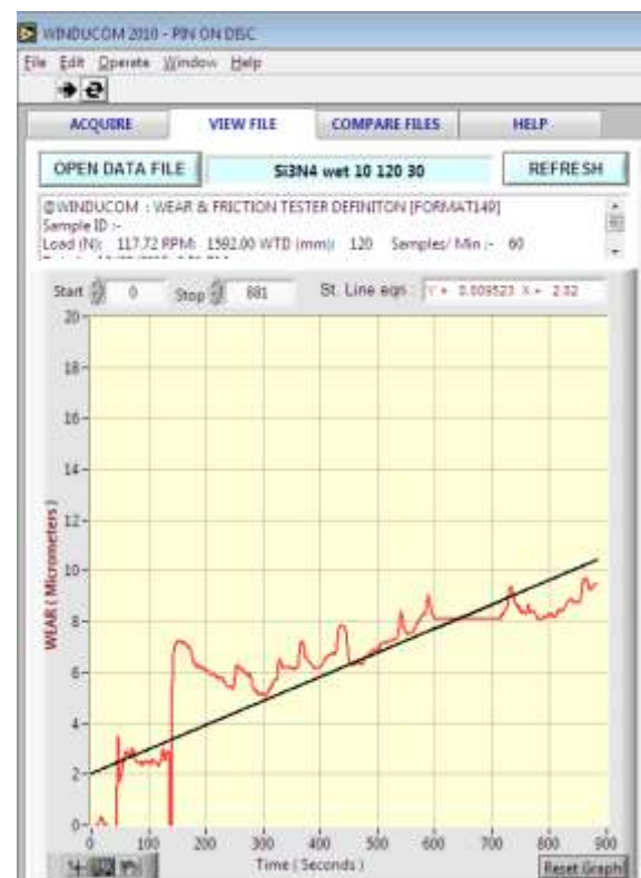
Figure 5 Wear V/s Time for Trial 2 with Alumina
